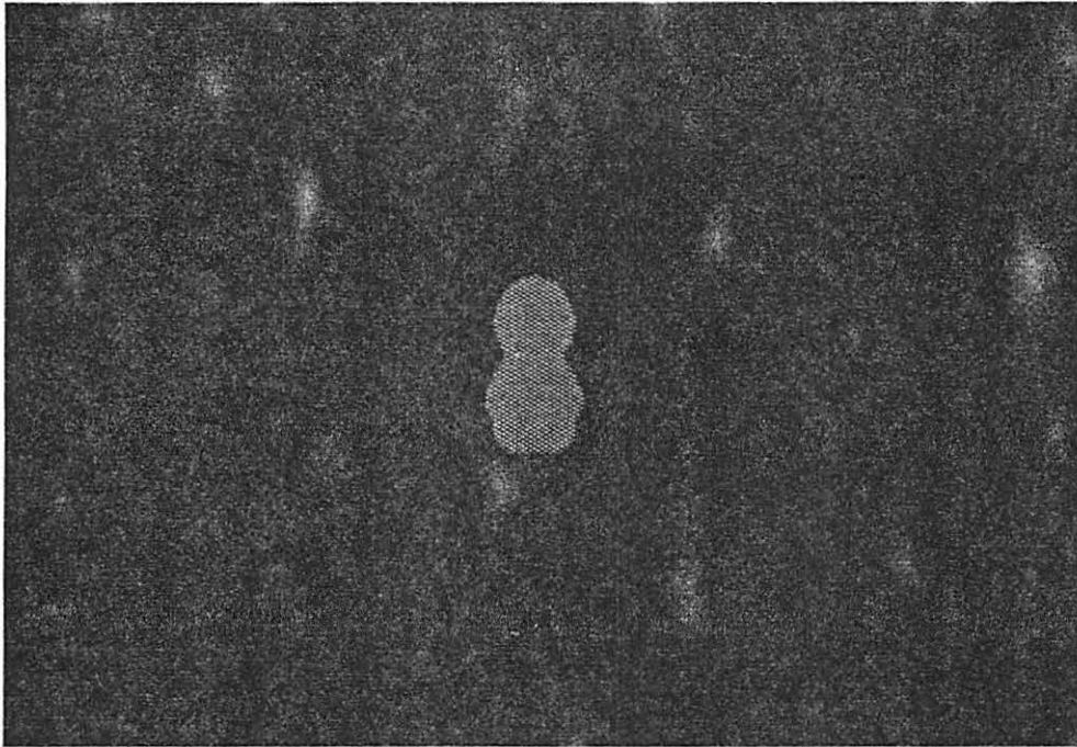
Figure 7.6: Simulated x-ray image of two flaws at different depths in the material
